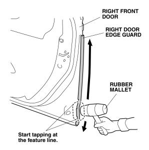
9. Repeat steps 3 through 8 to install the door edge guard on the left side of the vehicle.
